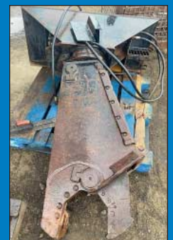
Asphalt Planner Grinder Skid
